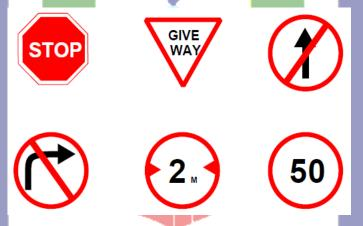
**Figure 2.9** Examples of regulatory signs (stop sign, give way sign, signs for no entry, sign indicating prohibition for right turn, vehicle width limit sign, speed limit sign)
