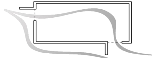
CROSS VENTILATION PLAN , wind wall size should be .5 - 1 x width of window
