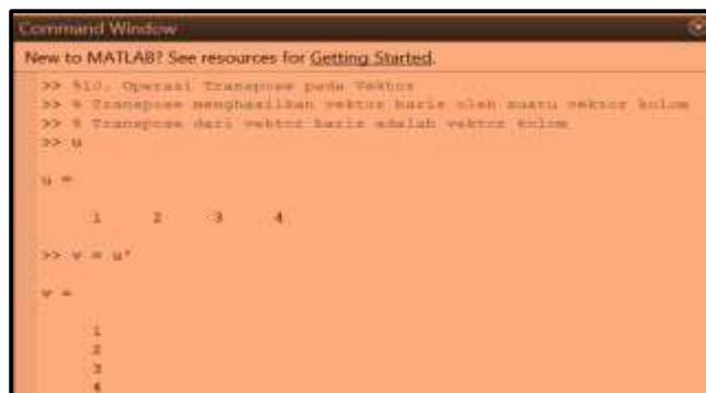
Gambar 3. 12. Operasi Transpose Vektor
