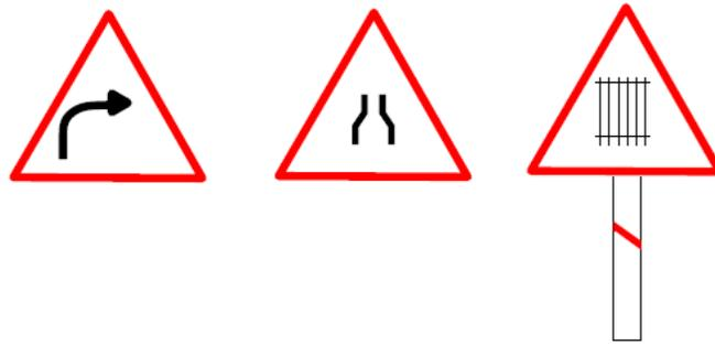
**Figure 2.10** Examples of cautionary signs (right hand curve sign board, signs for narrow road, sign indicating railway track ahead)
