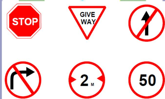
**Figure 2.9** Examples of regulatory signs (stop sign, give way sign, signs for no entry, sign indicating prohibition for right turn, vehicle width limit sign, speed limit sign)
